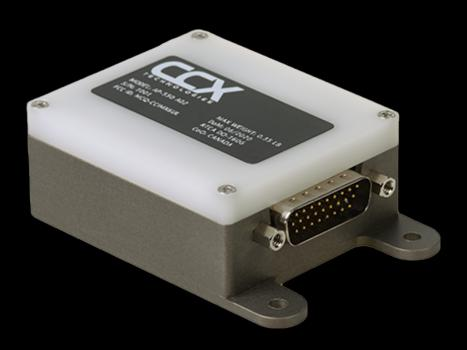
The AP-561 Micro-WAP is a small wireless access point that provides Wi-Fi connectivity to passengers and equipment onboard an aircraft. This small appliance can support up to five devices simultaneously, and offers additional cybersecurity and application hosting functionality.
