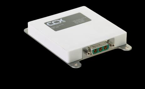
The IK-200 is a three element, dual-band Wi-Fi antenna designed for installation onboard an aircraft. This compact, directional antenna connects directly to the router/server and utilizes the IEEE 802.11 ac Wi-Fi standard to deliver enhanced signal strength to passengers and equipment onboard an aircraft. Connect up to two IK-200 Wi-Fi Antennas to any SystemX Appliance (AP-250/AP-251).
