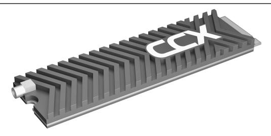
The EC-100 is a modern receive-only wideband software defined radio (SDR) M.2 Plugin Card that can support demanding security and connectivity tasks. This revolutionary SDR can receive frequencies up to 9 GHz, with a bandwidth of up to 800 MHz.
